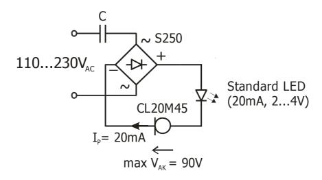
The circuit on the left simply needs 3 components to drive one (or more) Standard LEDs at a wide input range. The AC capacitor C has got a certain dynamic impedance  $X_C = 1/(2\pi fC)$ . Depending on the output power (and related to that, the input or mains current), there is a voltage drop across this impedance. C has to be chosen such way that the voltage drop is big enough to ensure that  $V_{AK}$  of the CLD is not exceeded.
