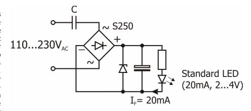
turn-on, a current peak can occur at the bridge, caused during initial charge of the AC and electrolytic capacitor. Therefore here the S250 by Diotec is used, featuring a very high forward surge rating of 40A (at 50Hz).
