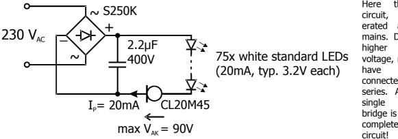
the same but operated at 230V<sub>AC</sub> mains. Due to the peak voltage, more LEDs to be connected series. Anyway, a rectifier bridge is enough to complete the whole circuit! The here
