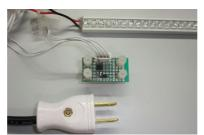
LED array driven at 110V<sub>AC</sub> by a bridge rectifier and a CLD
