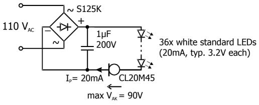
luminaire, operated at 110V<sub>AC</sub>, can be done. The here used Protectifiers® bridge S125K has the advantage of an increased ESD capability, and provides as such additional protection for the LED array.
