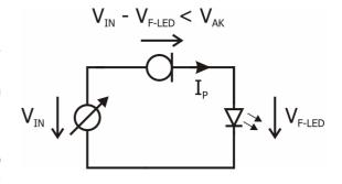
**to 90V\_{DC}.** For higher driving currents, the **CL40Mxx** offers an  $I_P$  of 40mA. CLDs can be even operated in parallel; of course then the power dissipation / power losses will increase as well.
